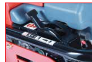
Two-In-One Lever and Kill-Switch interlocking with Fuel Cut-Off Mechanism for Easy Reach
