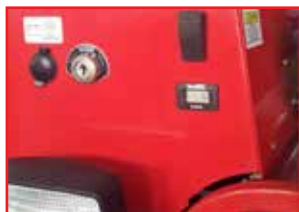
Light Switch, Key Switch, 12V Charger (To Charge Mobile Phones and Electronic Devices) and Tachometer Together in One Convenient Location.
