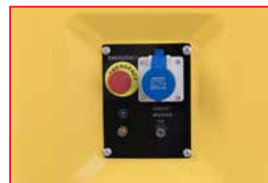
Simple design on control box with one power outlet socket
