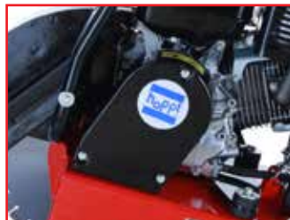
Belt Cover for Operators' Protection
