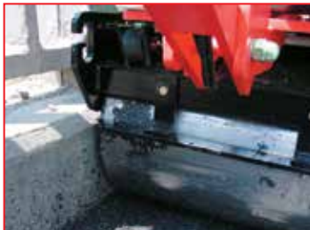
Low-Overhang for Compaction Right Up to the Edge of Curbside
